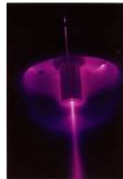
Electron beam produced by a pseudo-spark, © ONERA
