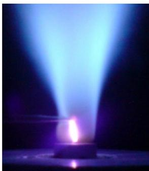
Fig. 1 Plasma-stabilized flame in a burner
