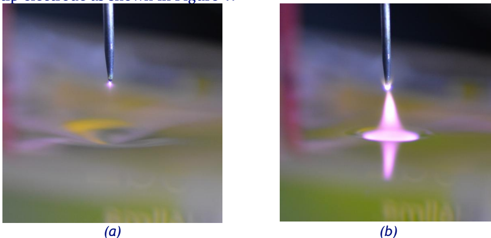
Figure 1. Photograph of a discharge between a high voltage tip and a grounded liquid: (a) corona discharge regime and (b) glow regime
